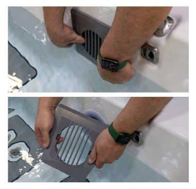
**Step 3:** Remove the filter basket assembly by gripping the basket handle and pulling outward.
