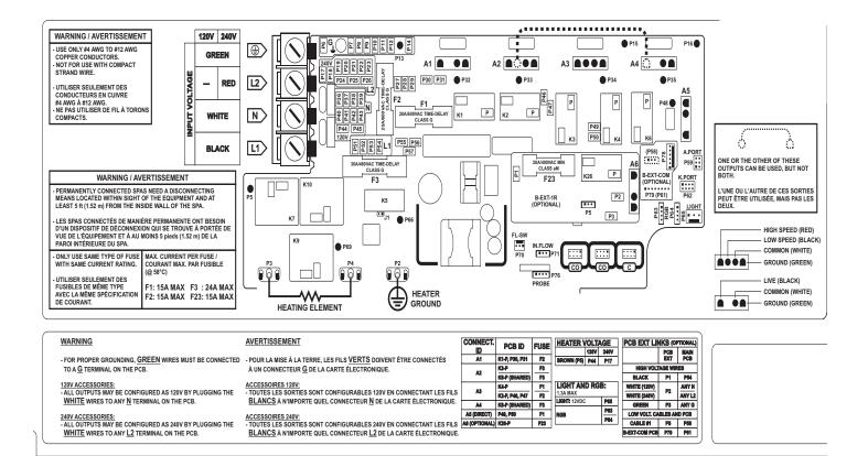
**NOTE:** Spa models with 3 jet pumps (S200) require a 60A service for full functionality. These models may alternatively be operated with various electrical configurations, however, certain set ups may result in operation limitations.
