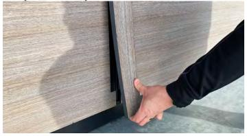
**Step 2:** Remove door - Carefully pull bottom of door out toward you. Carefully grab the bottom corner of the door and pull it out enough that you can slip your other hand in behind the side of the door about 4-5 inches (10-13 cm) up from the bottom. From there you will pull the door firmly away from the spa until the snap on the door pulls out of the snap feature in the rib. Continue to pull the door can then be dropped out of the groove on top and removed from the spa.
