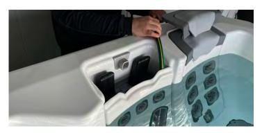
**Step 3:** Fill to the water level indicator or the mid point of the filter intake grate and proceed to start up procedure.
