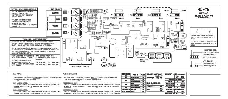
Insert each wire into the appropriate socket of the main entry terminal block according to the color code indicated on the sticker. Use a flat-head screwdriver to tighten the screws on the terminal.
