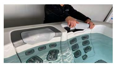
**Step 3:** While applying pressure downward on the manifold push the manifold toward the inside of the spa to release the manifold from the wall clip assembly, then lift the jet plate straight up to remove.
