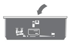
5 Use pliers on the wings of the clips, loosen from neck and flanged connector, slide up the hoses
