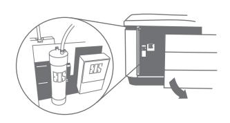
O Pull off the top and bottom hoses using a direct up or down motion
