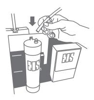
Replace left corner, tapping the cabinet to pop into the channels on the studs
